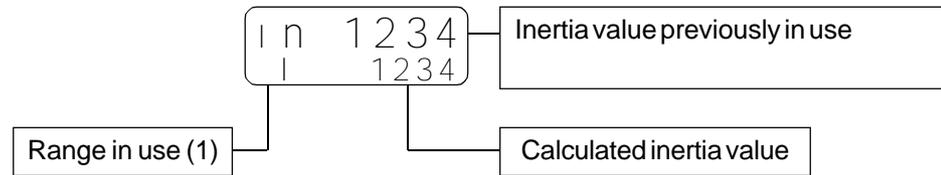
**P)** After the inertia value is confirmed with "ENTER", the instrument will display the tolerance activation delay time (the installer will choose whether to confirm or modify this value). After the "TA" parameter is confirmed with "ENTER", the instrument will automatically exit from the inertia calculation function.
