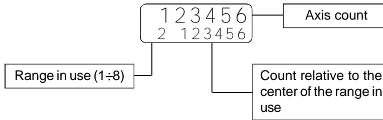
R) After the "**ENTER**" key has been pressed, the instrument positions the axis for the inertia calculation relative to the second range. This is carried out by repeating points M, N, O. Proceed with inertia calculation for all eight ranges.
